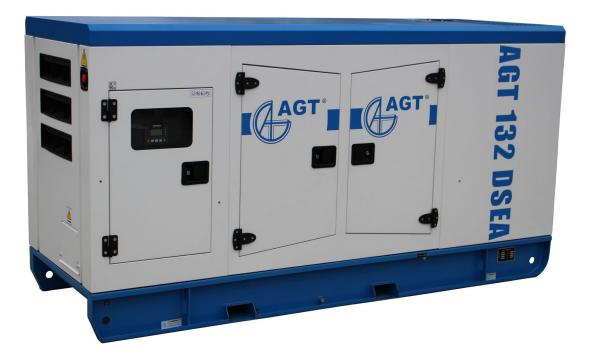
Voltage: Power factor: Max. power: Speed: Engine: Engine power: Displacement: Fuel: Alternator: Fuel tank capacity: Authonomy: Starting system: Protection degree: Overall dimensions: Weight: 400V / 50 Hz 0.8 127 kVA 1.500 rpm diesel, 4 cylinders, liquid cool 166 HP 6490 cm <sup>3</sup> diesel synchronous, AVR, brushless 240 l 12 h at 115 kVA load electric IP 23 2920mm × 1070mm × 1520mm 1680 kg
