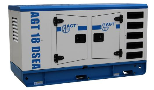
Voltage: Power factor: Max. power: Speed: Engine: Engine power: Displacement: Fuel: Alternator: Fuel tank capacity: Authonomy: Starting system: Protection degree: Overall dimensions: Weight: 400V / 50 Hz 0.8 18 kVA 1.500 rpm diesel, 4 cylinders, liquid cool 29.5 HP 2156 cm <sup>3</sup> diesel synchronous, AVR, brushless 25 l 8 h at 16 kVA load electric IP 23 1780mm × 770mm × 980mm 590 kg
