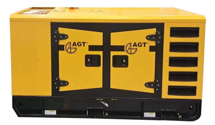
Voltage: Power factor: Max. power: Speed: Engine: Engine power: Displacement: Fuel: Alternator: Fuel tank capacity: Authonomy: Starting system: Protection degree: Overall dimensions: Weight: 400V / 50 Hz 0.8 33.0 kVA 1.500 rpmdiesel, 4 cylinders, liquid cool 44 HP  $3875 cm^3$ diesel synchronous, AVR, brushless 80 I 11.5 h at 30 kVA loadelectric IP 23  $2050mm \times 1000mm \times 1255mm$ 970 kg
